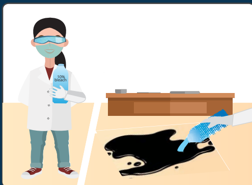
Pour freshly made 10% bleach on absorbent materials in a spiral motion, starting from the outside of the spill working your way into the center.
