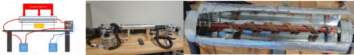
Figure 2: (Left) Schematic of Test Bench Setup (Center) Built Test Setup (Right) Internals of Casing
